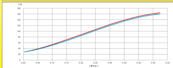
Variation, as a function of the power in W/cm<sup>2</sup> of the silicone heating ribbon, of the wall temperature of an empty, galvanized steel tube, thermally insulated by 20mm PVC-NBR foam
