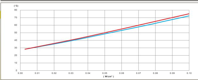
Variation, as a function of the power in W/cm² of the silicone heating ribbon, of the wall temperature of an empty PVC tube, thermally insulated by 20mm of PVC-NBR foam
