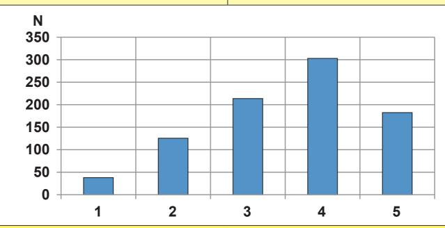
Comparative tear strength of the different thicknesses models 1: 0.8mm; 2: 1.6mm; 3: 2.3mm; 4: 3.2mm; 5: 2.3mm with stainless steel mesh reinforcement
