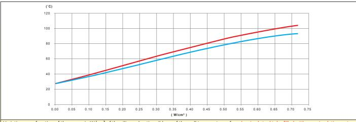
Variation, as a function of the power in W/cm<sup>2</sup> of the silicone heating ribbon, of the wall temperature of a galvanized steel tube filled with non-circulating water, non-thermally insulated
