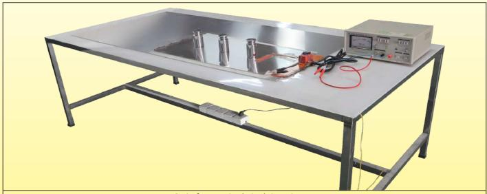
Device for measuring the insulation resistance.
