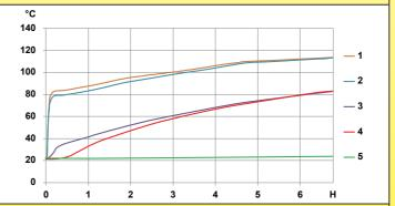
1: Surface temperature between silicone belt and drum 2: Outside silicone belt surface temperature
