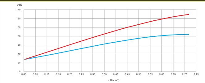
Variation, as a function of the power in W/cm<sup>2</sup> of the silicone heating ribbon, of the wall temperature of a PVC tube filled with non-circulating water, non-thermally insulated
