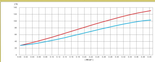
Variation, as a function of the power in W/cm<sup>2</sup> of the silicone heating ribbon, of the wall temperature of a PVC tube filled with non-circulating water, thermally insulated by 20mm PVC-NBR foam
