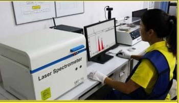
Spectrometric analysis in progress (Ultimheat Laboratory)
