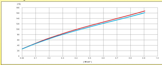
Variation, as a function of the power in W/cm² of the silicone heating ribbon, of the wall temperature of an empty, non-thermally insulated galvanized steel tube
