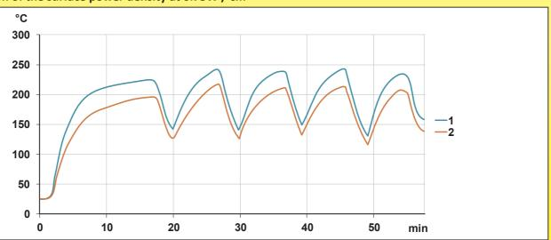
Temperature measurement made on a 200mm width silicone belt mounted on a 55 gallons (200 liters) drum. Power 2250W (0.75W/cm²), PID controller with sensor located in the center of the empty tank. Surface temperature limited to 190°C by a disc thermostat.
